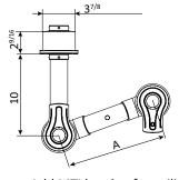
Add MTI bracket for ceiling mounting. Add MVK bracket for wall mounting.
