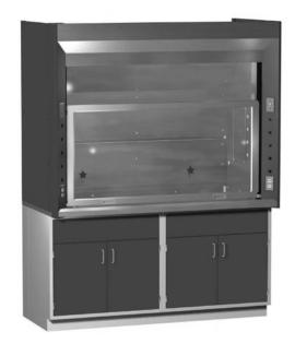
\*SPECIAL NOTES: Perchloric hoods attached to long runs of ductwork require solenoid activated, electronically sequenced spray head activation to assure the flow rate into the fume hood washdown trench never exceeds the 45 GPM overflow rate. Any blower purchased to exhaust this hood should have internal washdown capability and be lubricated with fluorocarbon grease and oil.
