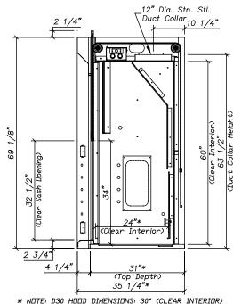
NDTE: D30 HODD DIMENSIONS: 30° (CLEAR INTERIOR) 37° (TOP DEPTH) / 41 1/4° (D.A. DEPTH)
